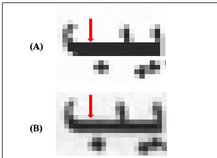
Figure (4.7): (A) Edge Gradient for fabricated text. (B) Edge Gradient for non-fabricated text
