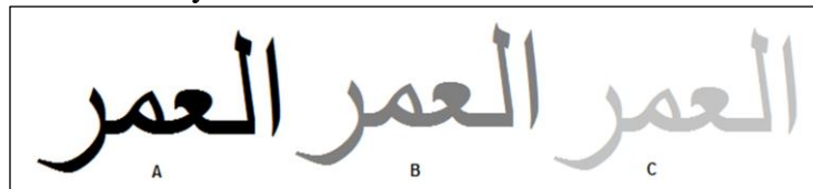
Figure (4.4) Example of gray level of intensity, where intensity of (A) is 0, (B) is 127, and (C) is 195.
